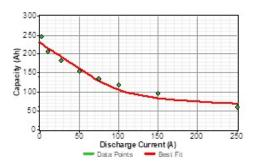
Figure 4: The capacity curve of Trojan T-105 Battery.
