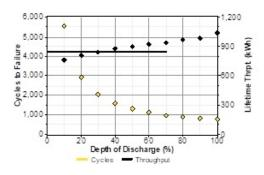
Figure 5: The lifetime curve of Trojan T-105 Battery.
