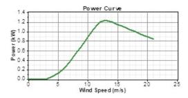
Figure 3: The power curve of BWC XL.1 wind turbine.
